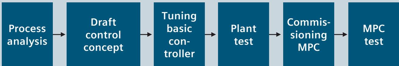
Simplified procedure for the implementation of the MPC controller
