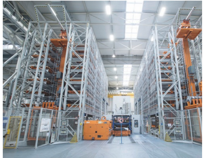
Automated guided vehicles (AGVs) deliver metal blanks to the loader of the press line, where they are processed further.
