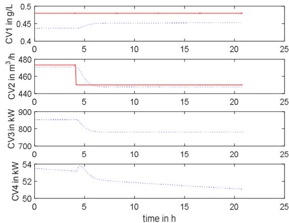
Figure 9: Setpoint step in permeate flow (CV2) – trend of controlled variables. For CV1 the red line shows the upper limit of salinity i.e. salinity is inside its control zone all the time. For CV2 the red line is the permeate flow setpoint. CV3 and CV4 have setpoints below the axis limits and low priority.
