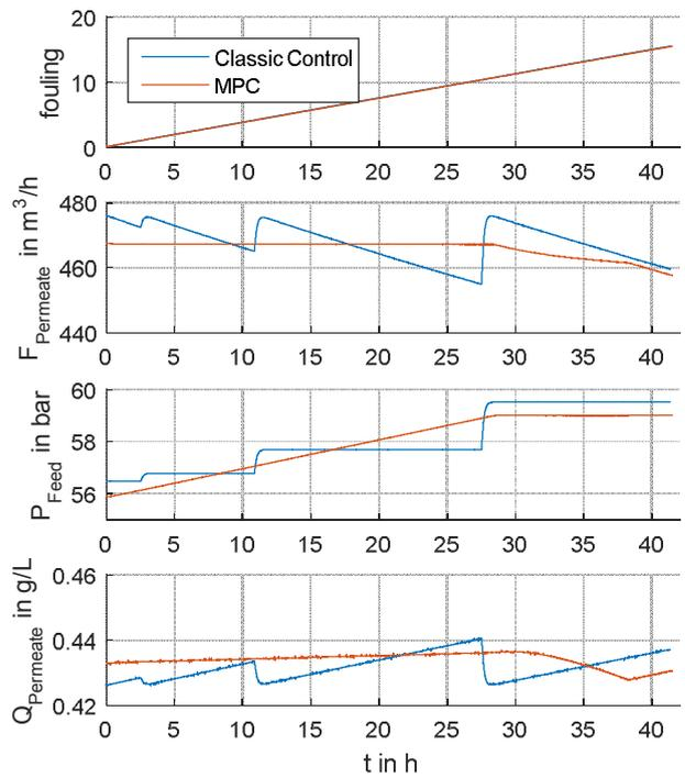
Figure 13: Benchmarking simulation, blue: classic control, red: MPC. From top to bottom: fouling, permeate flow (CV2), feed pressure (MV1), permeate salinity (CV1)
