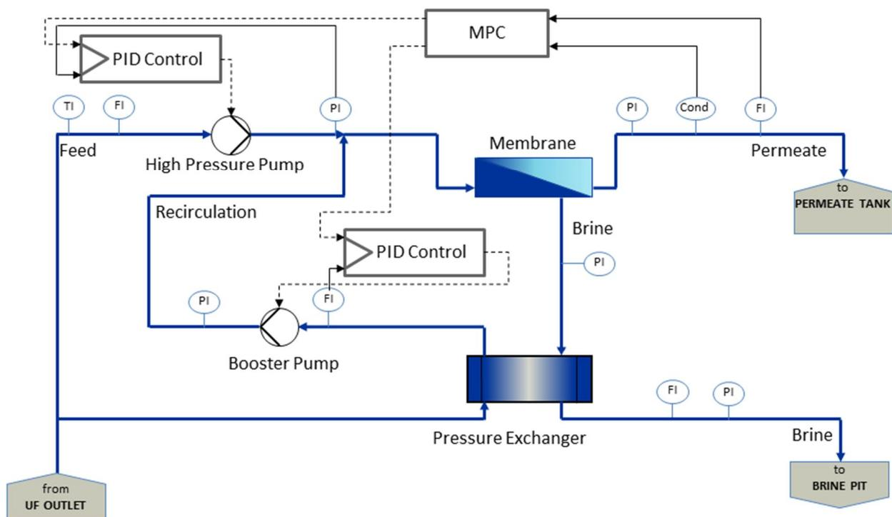
Figure 8: P&I diagram of reverse osmosis unit with MPC
