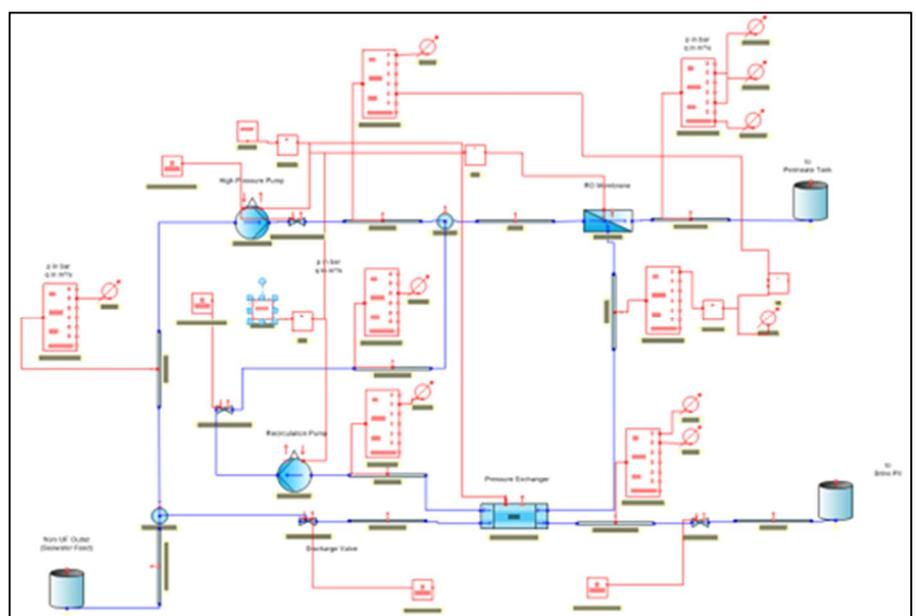
Figure 5: Simulation model of reverse osmosis unit
