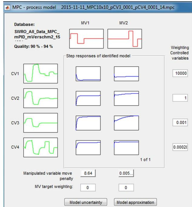
Figure 6: MPC configurator session with process model and weightings
