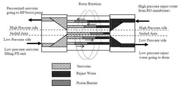
Figure 4: Schematics of rotary pressure exchanger [11.]
