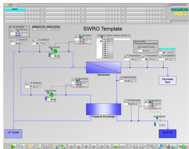
Figure 7: Simatic PCS 7 OS picture of membrane unit template
