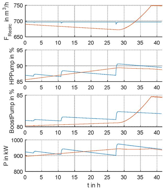
Figure 14: Benchmarking simulation, further variables from top to bottom: recirculation flow (MV2), high pressure pump speed (CV3), booster pump speed (CV4), overall electric power consumption of both pumps
