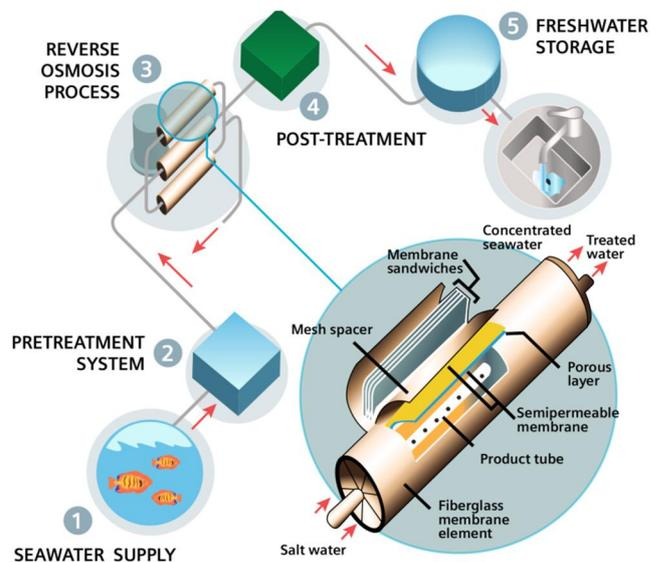
Figure 1: Overview of reverse osmosis seawater desalination process
