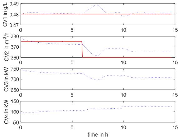
Figure 11: Setpoint step in permeate flow while salinity is at its limit – trend of controlled variables. CV1 salinity has higher priority than CV2 permeate flow. Therefore the limit violation of salinity is compensated while some deviation in permeate flow is tolerated.
