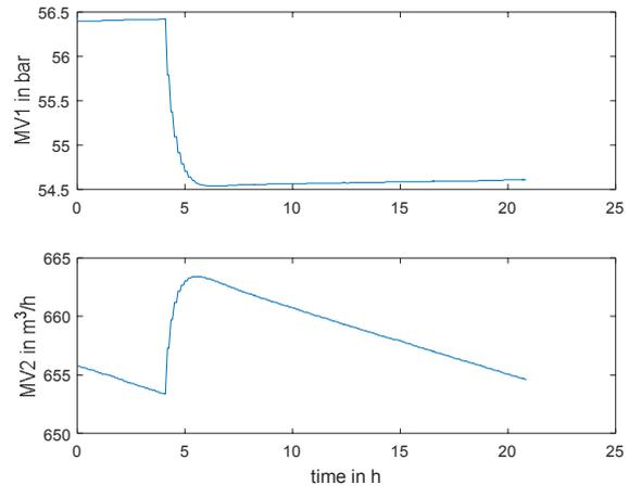
Figure 10: Setpoint step in permeate flow (CV2). The trend of manipulated variables shows that the MPC uses both of them in a coordinated way to reach the new setpoint
