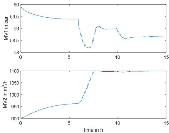
Figure 12: Setpoint step in permeate flow while salinity is at its limit – trend of manipulated variables
