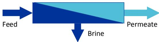
Figure 2: Schematic view of reverse osmosis membrane
