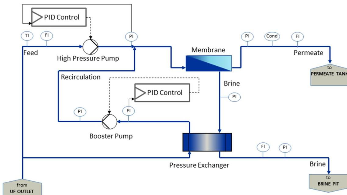
Figure 3: P&I-diagram of reverse osmosis unit with conventional automation
