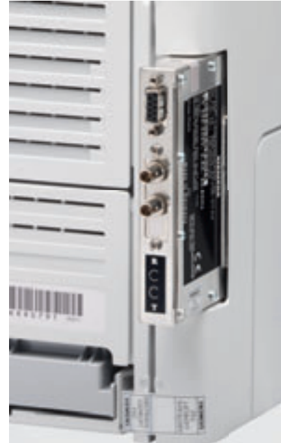
Filtered connections make the SITEMP printer spy-proof
