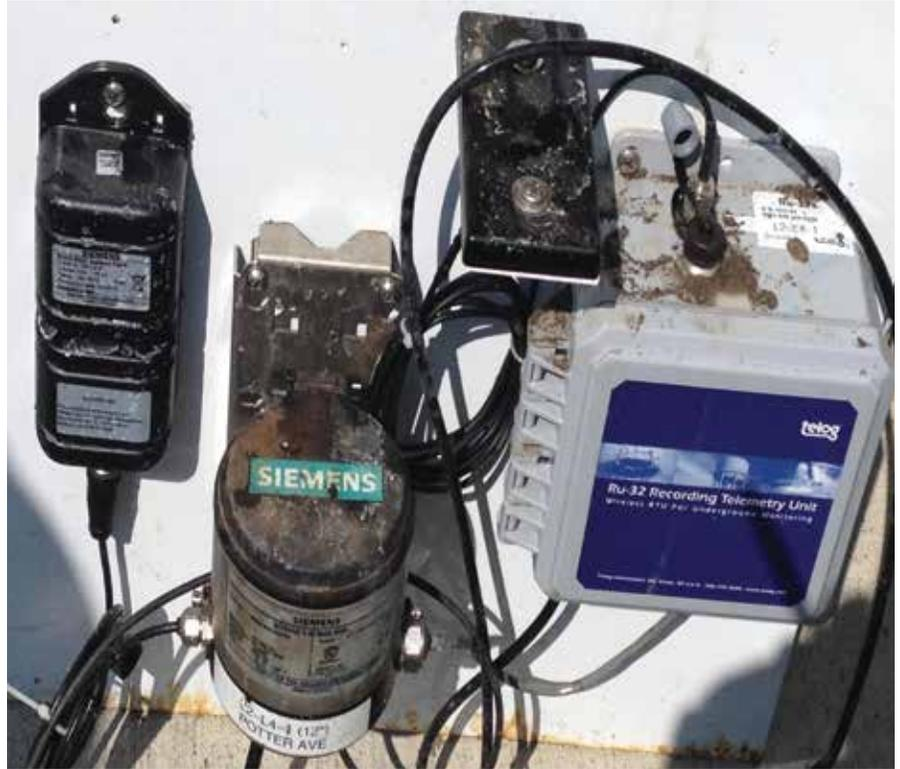
Figure 4 Flow transmitter, battery, data logger and modem
