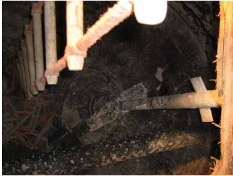
This process vessel contains an agitator – an obstruction that makes continuous level measurement a definite challenge.
