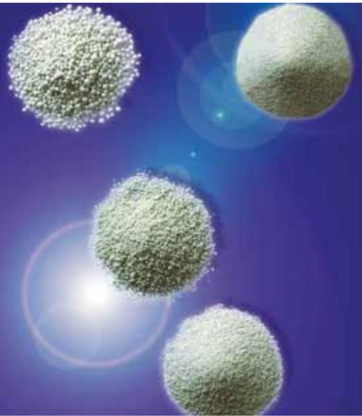
Poraver North America produces this unique, light-weight aggregate in a variety of sizes, all made from post-consumer glass.
