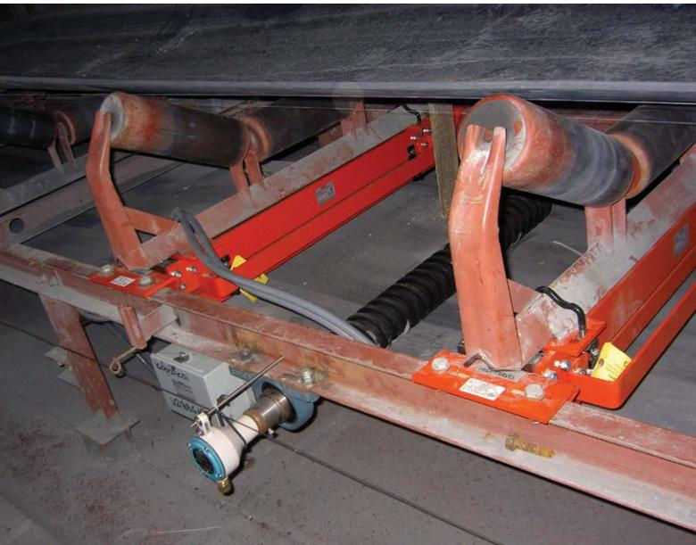
Technicians at the minerals processing plant installed the Milltronics MMI belt scale and SITRANS WS300 speed sensor easily and quickly.
