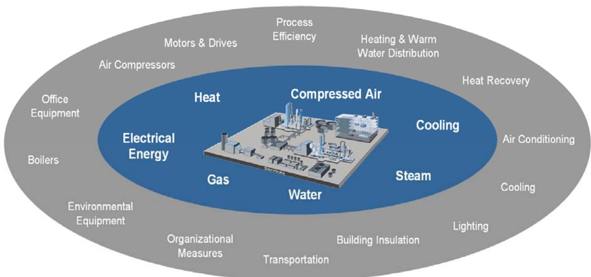
Fig. 3-2: Forms of energy and energy management topics in a process engineering production plant
