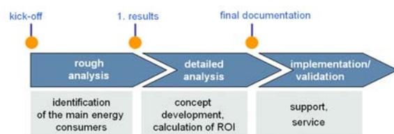
Fig. 5-1: Typical sequence of process engineering energy optimization
