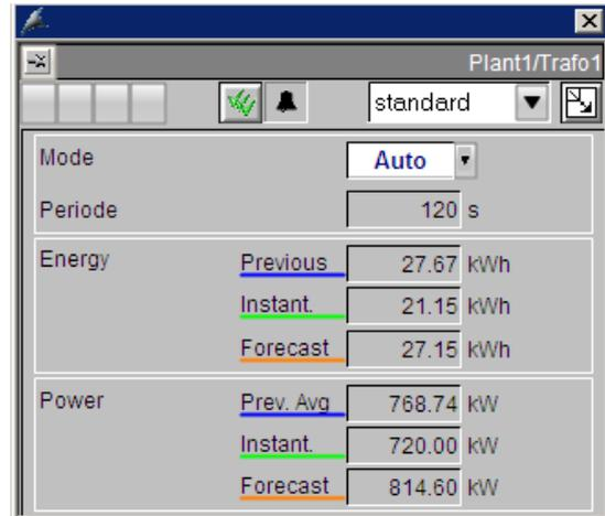
Fig. 4-3: PCS 7 faceplate of SIMATIC powerrate for one power consumer
