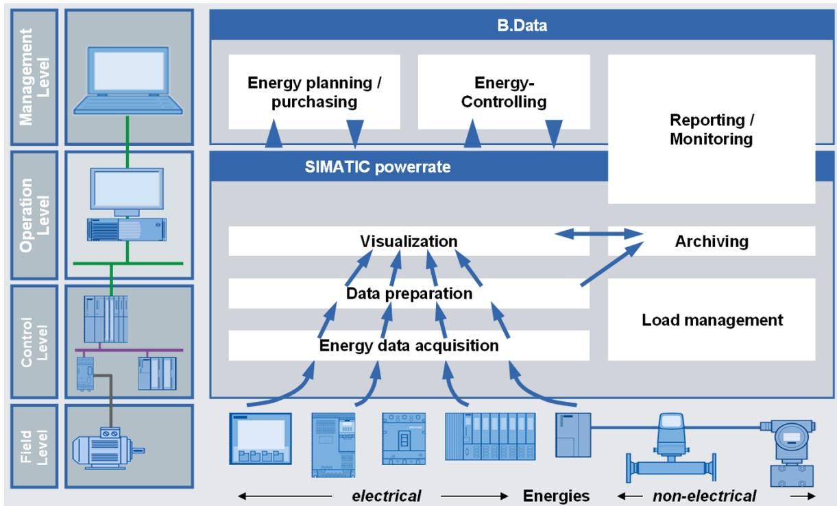
Fig. 4-1: Standard components for energy efficiency and energy management
