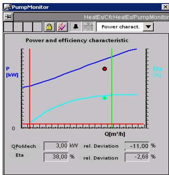
Fig. 4-7: Faceplate of the PCS 7 PumpMon function block with characteristics curves for mechanical shaft power and hydraulic efficiency dependent on flow
