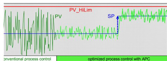
Fig. 4-6: Optimized process operation with Advanced Process Control (APC)
