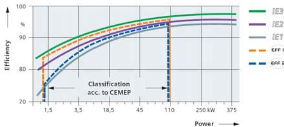
Fig. 4-10: Efficiency factors of electric motors; Source: [20.]
