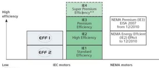
Fig. 4-9: New efficiency classes for electric motors according to IEC 60034-30
