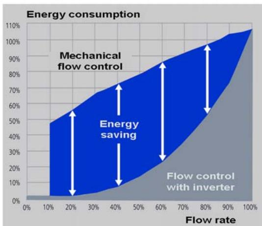
Fig. 4-8: Energy saving by using speed-controlled pumps instead of throttle valves
