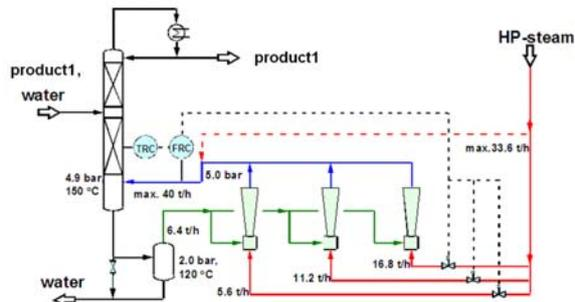
Fig. 5-2: Use of a steam jet to reduce the high-pressure steam demand during separation of water and product 1
