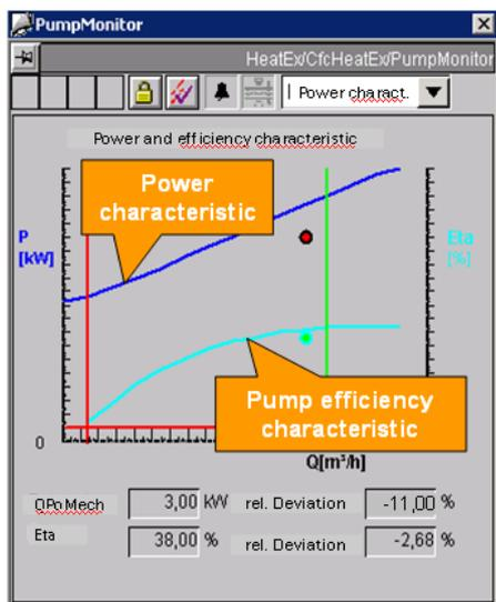
Picture 5: Power characteristic and efficiency characteristic with current operating points
