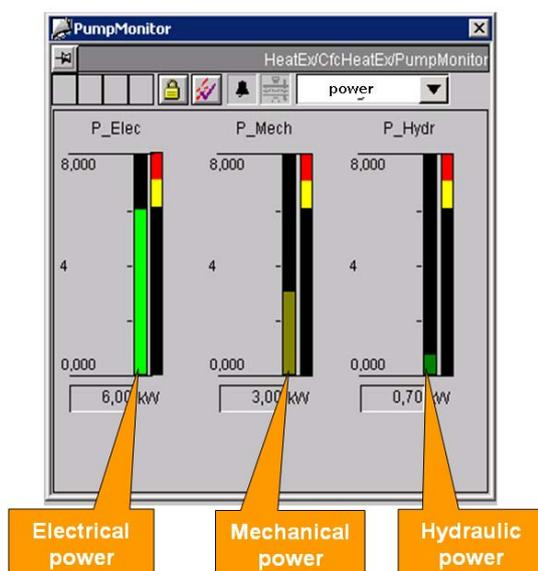
Picture 3: Power values with alarm limits
