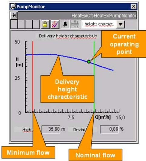
Picture 4: Delivery height characteristic with „live“ operating point
