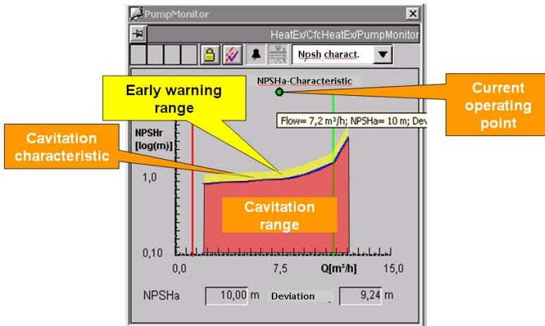
Picture 6: NPSH characteristic with current NPSHa value
