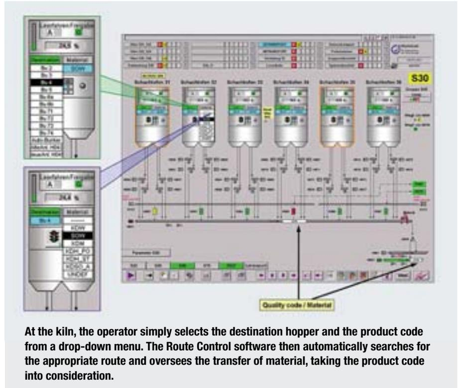
**At the kiln, the operator simply selects the destination hopper and the product code from a drop-down menu. The Route Control software then automatically searches for the appropriate route and oversees the transfer of material, taking the product code into consideration.**
