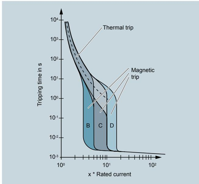
Fast tripping is important, because when the 24 V DC supply fails the intact branches are also undersupplied. Voltage interruptions of 20ms are already critical for the PLC and will cause the process to be interrupted or even to crash.
