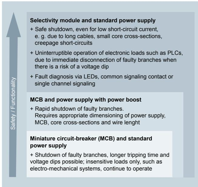
Switched mode power supplies with miniature circuit-breakers offer a cost-efficient solution for loads that are not affected by voltage drops.
