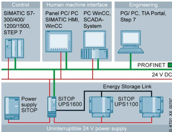
Figure 8: Backing up an automation solution with PLC networked via PROFINET. Even multiple controllers can be brought to a defined state independent of each other
