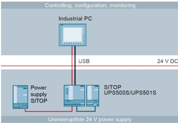
Figure 5: Backing up a 24 V automation computer with communication via USB
