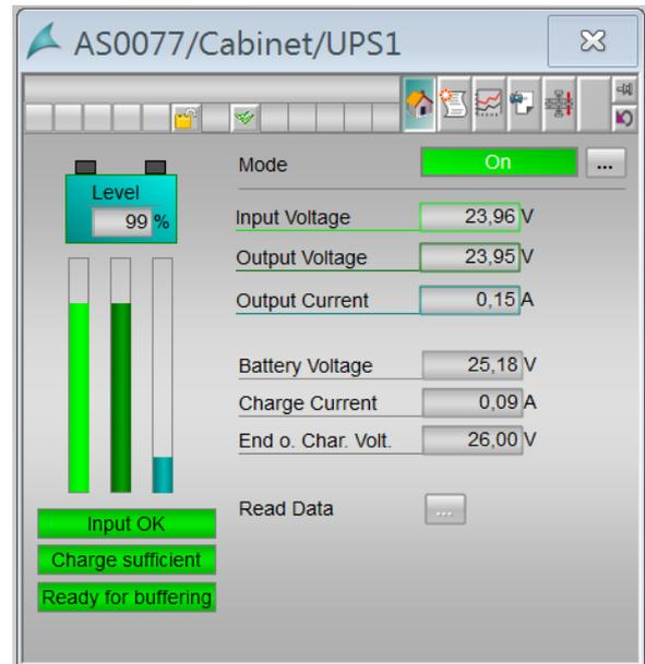
Figure 10: Faceplates for the SIMATIC PCS 7 enable easy diagnostics and maintenance of the DC UPS in the process industry
