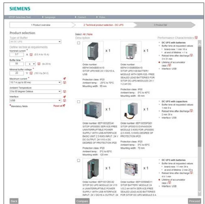
Figure 3: After entering a few criteria, the SITOP Selection Tool offers a selection of suitable DC UPS configurations.
