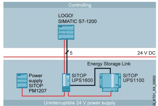
Figure 4: Backing up simple automation applications with status signaling via digital outputs.
