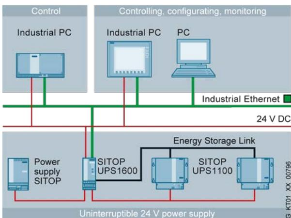
Figure 6: Backing up multiple 24 V PCs. Communication via Industrial Ethernet supports comprehensive diagnostics and targeted shutdown in the master-slave module in case of power failure
