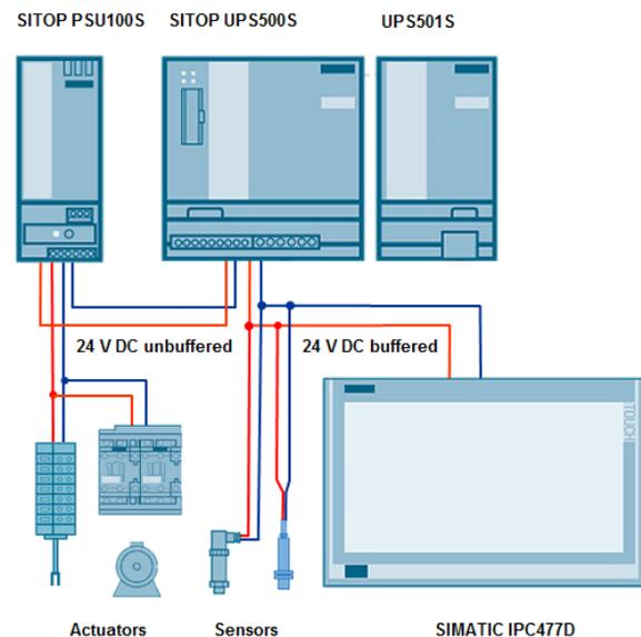
Figure 2: Application example for configuration of an uninterruptible 24 V power supply
