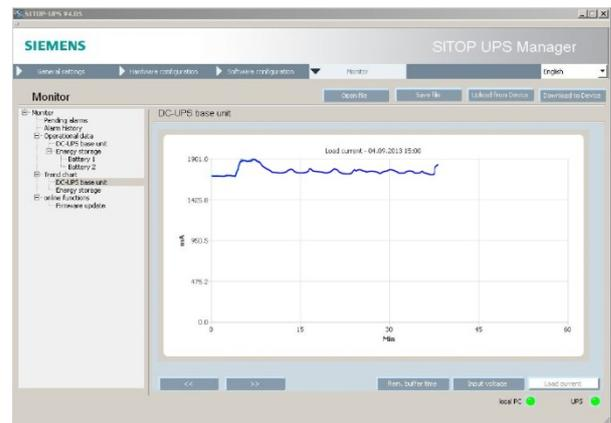
Figure 7: The various trend charts of the SITOP UPS Manager support comprehensive diagnostics of the network status and the status of the DC UPS.
