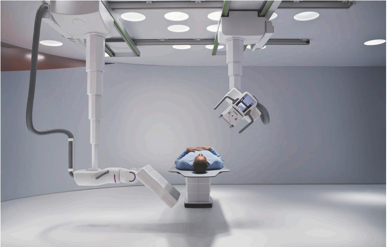
Siemens Healthineers relies on wireless LAN in various X-ray machines. The wireless communication technology is fully integrated into the X-ray detectors. The image depicts a stationary device, the world's first twin-robotic X-ray scanner Multitom Rax.
