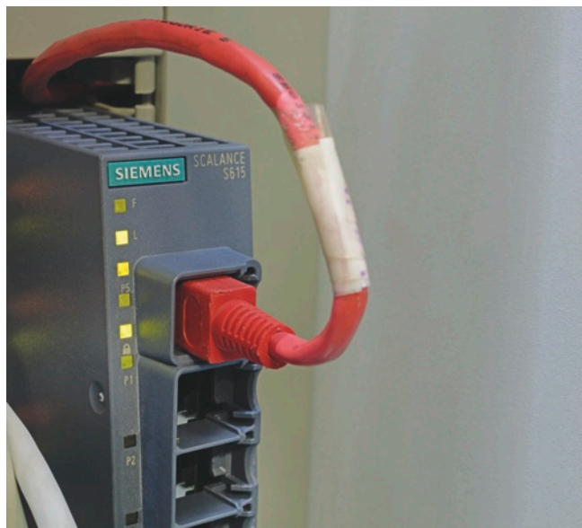
The interface to Simema Remote Connect at ACSR are the SCALANCE S615 Security Modules, which could be integrated reactionless into the operator network.
