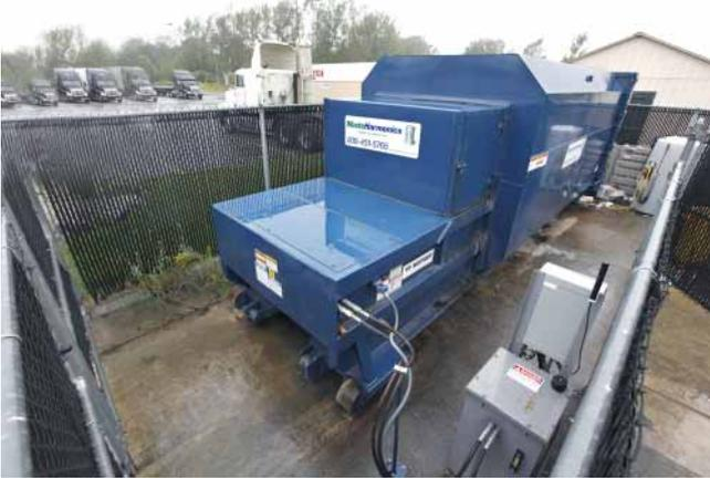
Trash compactors are designed for extreme weather and operating conditions. Thanks to the telemonitoring by means of standard components from Siemens, Waste Harmonics can keep an eye on many operating parameters – cost-effectively and independent of the location. This enables predictive maintenance and fast troubleshooting.
