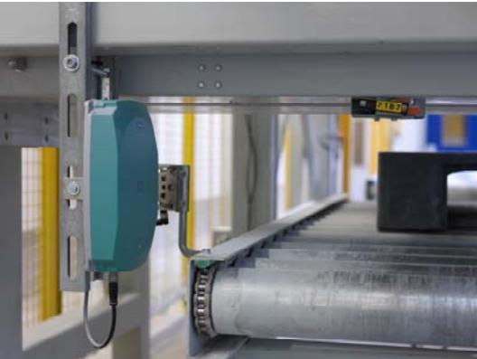
The compact design of the UHF reader SIMATIC RF620R enabled an easily accessible installation for cleaning and maintenance despite the restricted space conditions.
