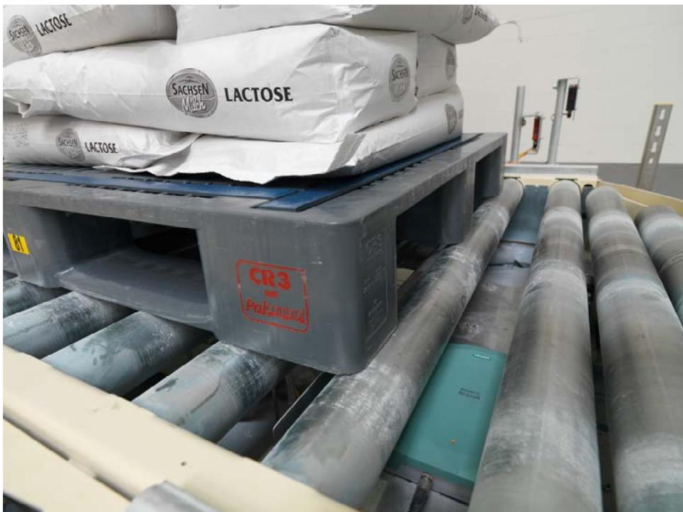
As soon as an RFID pallet passes the sensor, a time slot for the read operation is opened in the UHF reader, which is mounted below the roller conveyor.
