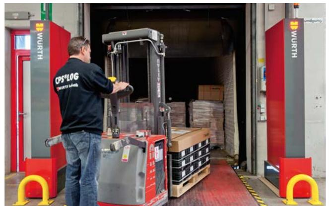
The RFID gate at the loading ramp is equipped with a reader SIMATIC RF670R and four detached antennas. Triggered by passing through a light barrier, the RFID data of the pallet is captured and transmitted to the enterprise resource planning system (ERP).
