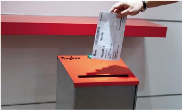
The iTagbox is designed for pallet Kanban with bulky parts. Comparable to a mailbox, dropping in Kanban cards with RFID tags signal the goods requirement. The antenna of the iTagbox is connected directly to the RFID reader of the pallet box.
