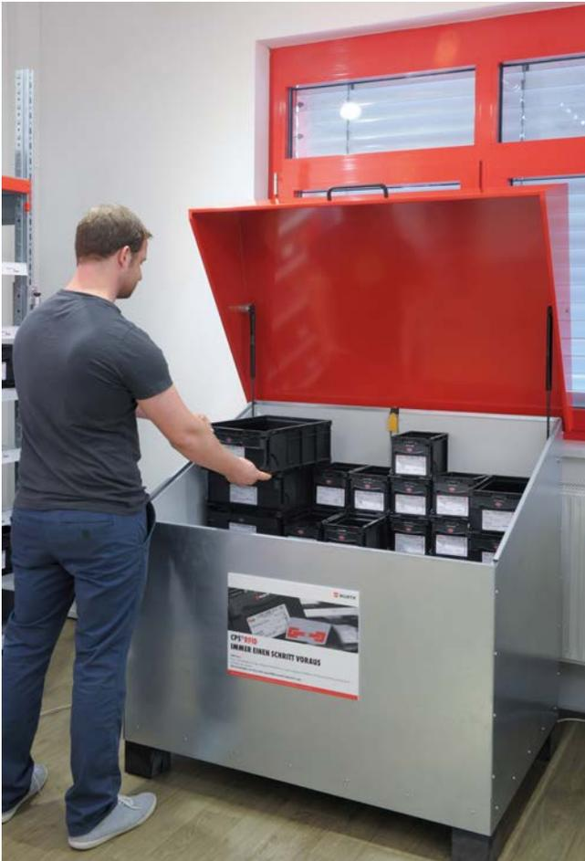
The RFID pallet box (iBox) is the centerpiece of the Würth logistics solution. As soon as an employee places the empty small parts container into the iBox and closes it, ...
