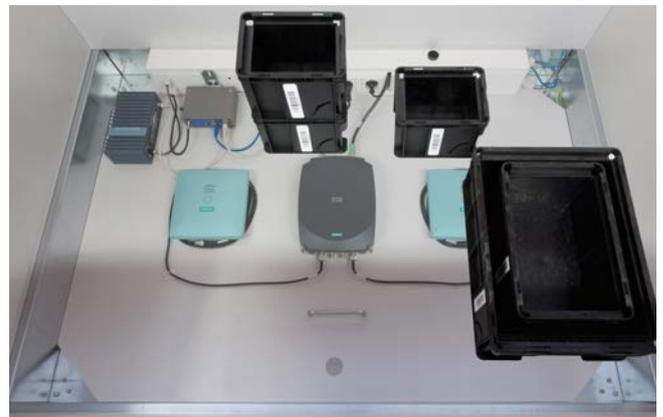
... a reader SIMATIC RF670R with two detached UHF antennas SIMATIC RF640A captures the tag data and transmits it from the customer to the Würth logistics center.
