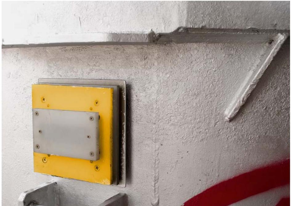
The high external temperatures are dissipated to the ambient air through a multilayered design so that the SIMATIC RF620T transponder (below the white cover plate) is operated within the specification.
