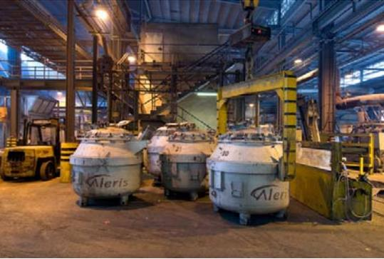
The aluminum is transported in molten state in specially insulated crucibles
