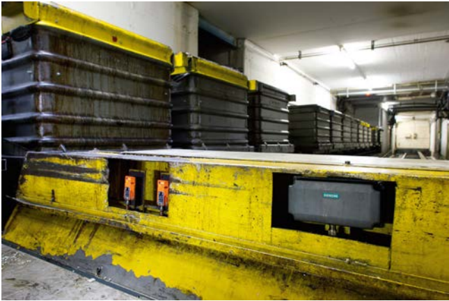
Image 4: The SIMATIC RF380R RFID reader reads the bin numbers stored on the transponders and guides the bins in the right direction
