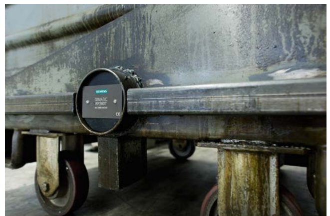
Image 3: All 23 lorries are equipped with a SIMATIC RF360T RFID transponder, which enables a clear recording and assignment of materials and weights
