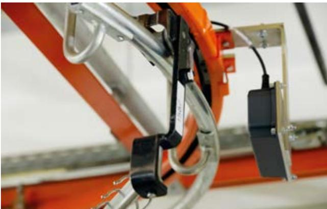
Simple to install, rugged and cost-efficient: Mobile data carrier SIMATIC MDS D160 (on the left) in the spacer on a trolley. The read distance to the SIMATIC RF380R reader (on the right) can be up to 80 mm
