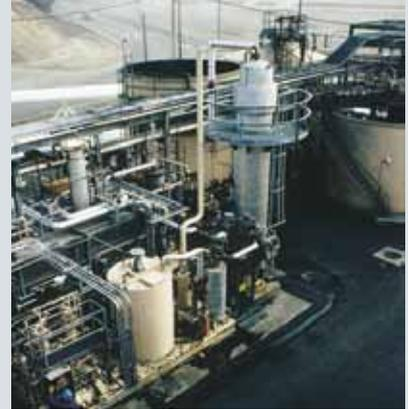
*The wet air oxidation process is used to destroy biological solids and regenerate carbon at a Tosco refinery. In this application, the wet air oxidation process is referred to as the wet air regeneration process.*
