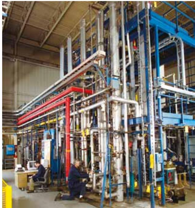
*Our pilot testing facility is the largest of its kind in the world with numerous pilot units constructed of various alloy materials.*
