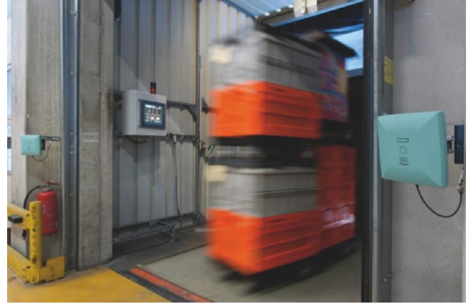
Image 2: Two RFID antenna pairs, activated by motion sensors, contactlessly read the transponders/tags on the dollies and in doing so recognize the correctness of the goods and the load direction
