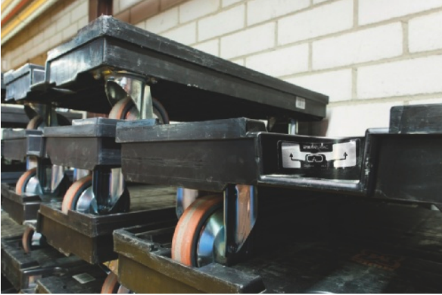
Image 3: The RFID tags SIMATIC RF630L are affixed protected to approximately 190,000 dollies and store their unique number
