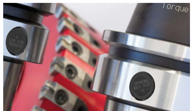
For the flush installation of the data media MDS D421, holes are drilled into the tool. The read/write distance is eight millimeters.
