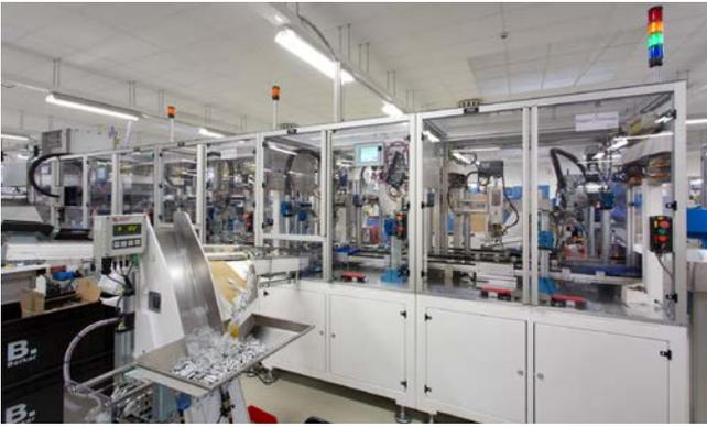
From Hager MD (Machinery Department) for Berker implemented, largely automated assembly and testing line Ecoline for channel-track sockets.
