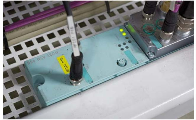
Via interface modules Moby ASM 456 and PROFIBUS, the SIMATIC readers RF240R are connected to the failsafe line controller SIMATIC S7-300F.
