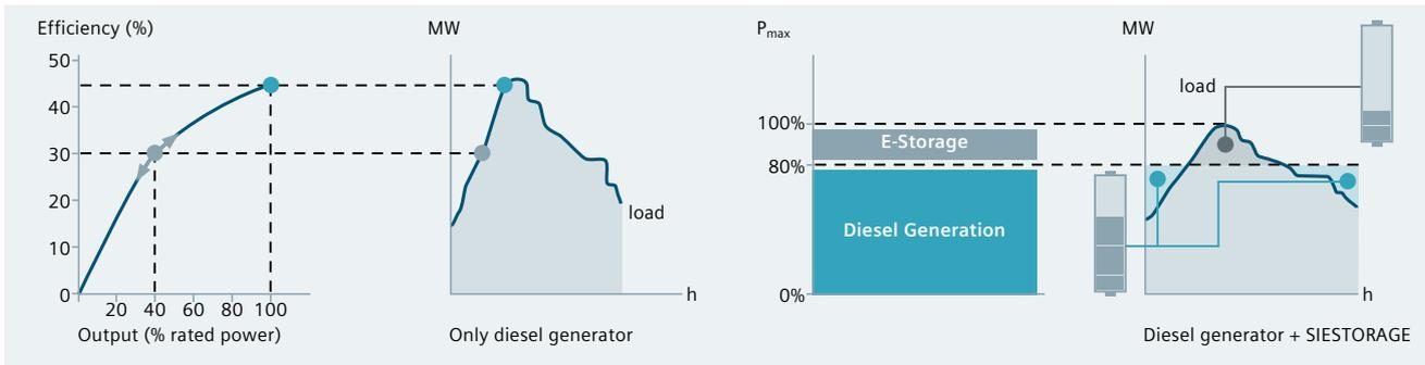
Example of how SIESTORAGE optimizes the diesel generator performance
