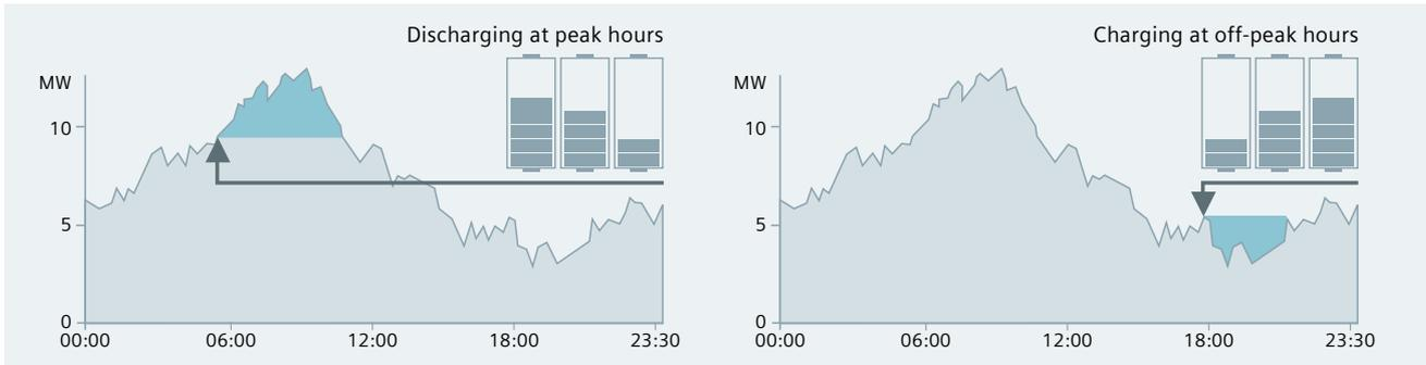
Example of how SIESTORAGE helps to improve peak load management and cost efficiency by balancing supply and demand
