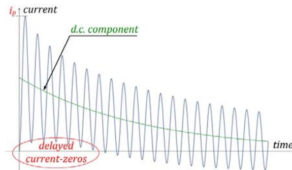
**Fig. 3** Short circuit current with delayed current zeros
