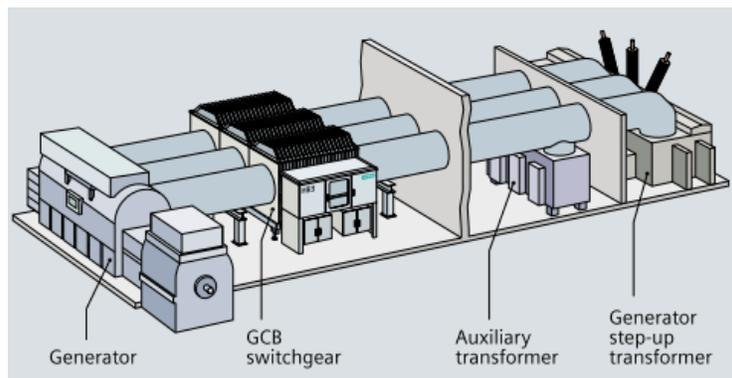
**Fig. 1** A typical layout of a generator circuit
