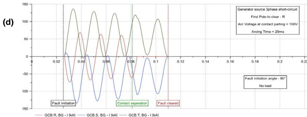
**Fig.8** Three phase generator fed fault current with the arc voltages of (a) 0V, (b) 30V, (c) 60V and (d) 100V
