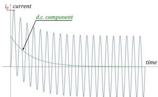
**Fig. 5** Short circuit current with higher magnitude
