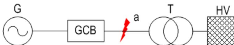
**Fig. 7** Simplified single line diagram of a generator circuit.
