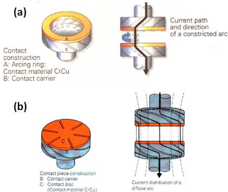
**Fig. 6** Types of vacuum interrupter contacts (a) RMF contacts, (b) AMF contacts.
