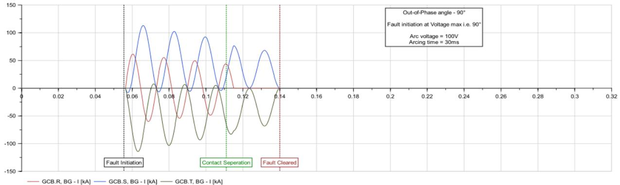
**Fig.9** Out-of-phase synchronizing at  $90^\circ$  with (a) without interruption (b) interruption with 0V arc voltage, (c) with 50V arc voltage and (d) with 100V arc voltage.
