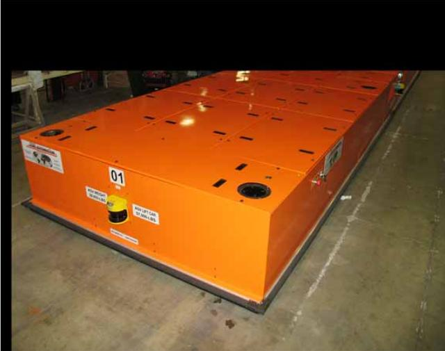
The AGV systems are specifically developed for the transport of large payloads and tooling through the production floor.
